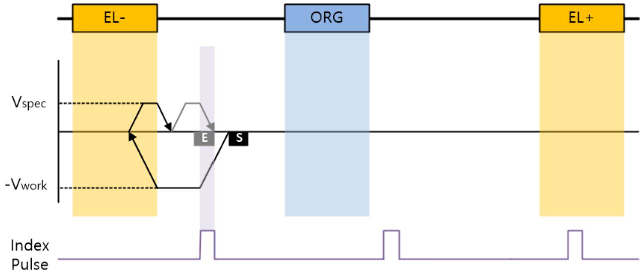
**EL ON → STOP → BWD(HS) → EL OFF → STOP → BWD(HS) → Z-Pulse ON → STOP**
