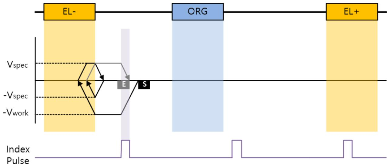
**EL ON → STOP → BWD(HS) → EL OFF → STOP → FWD(HS) → EL ON → STOP → BWD → Z-Pulse ON → STOP**
